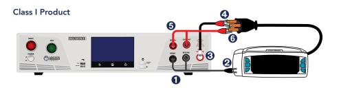
If there is no ground circuit present on the DUT, you can use test leads to connect the HypotULTRA $^{\otimes}$  to the DUT.
